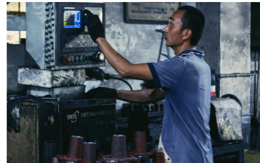
Pump Casing Drilling
